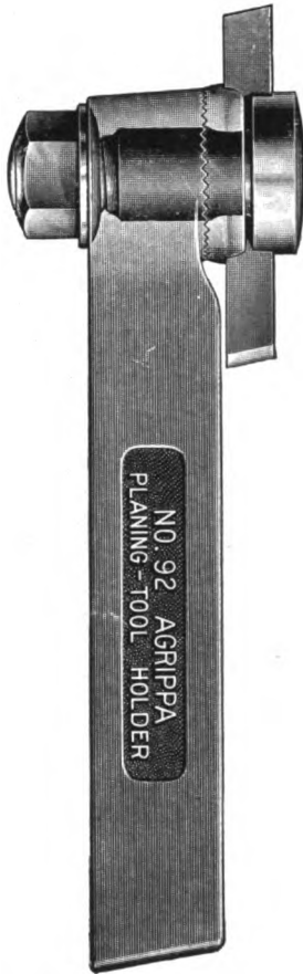
The Planing Tool has a serrated ring of improved steel which affords unequal variety and rapidity of adjustment. The ring is correctly hardened to resist the wear of the cutter. The body of the holder receives a very different heat treatment that prevents breakage.
